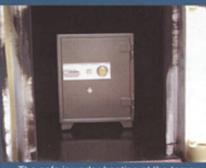
The safe is under heating at the temp. of 1,010 °c for 2 hours.
