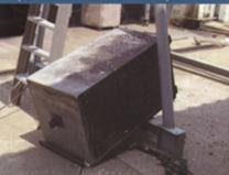
The safe is hoisted up to 4 m. above the concrete floor and then dropped.
